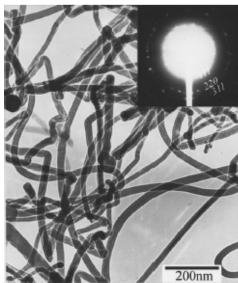
Fig. 10.21. A TEM image of Ge nanowires and a selected-area electron-diffraction pattern (inset) [35].
